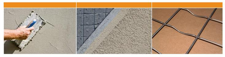
Structalath No. 17 SF CR II is a welded wire lath engineered to enhance the performance of stucco cladding. Structalath 316 is a modified version of our Structalath that features a reduced furr depth for use with 1/2" systems – with or without foam. The flat furr design ensures there will be no damage to the vapour barrier and promotes uniform thickness in a one-coat system. Structalath is easy to handle and improves construction site efficiency.
