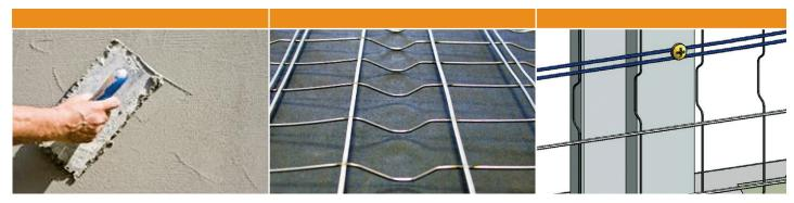
Structalath Twin Trac 316 is a self furring welded wire lath for use as an alternative to the 2.5 lb/yd² diamond mesh metal lath as specified in ASTM C 847 and for use as an alternative to the 1.14 lb/yd² welded wire lath specified in ASTM C 933. Structalath Twin Trac 316 is a version of Structalath Twin Trac that features reduced furr depth for use with 1/2" systems – with or without foam. The flat furr design ensures there will be no damage to the vapour barrier and promotes uniform thickness.
