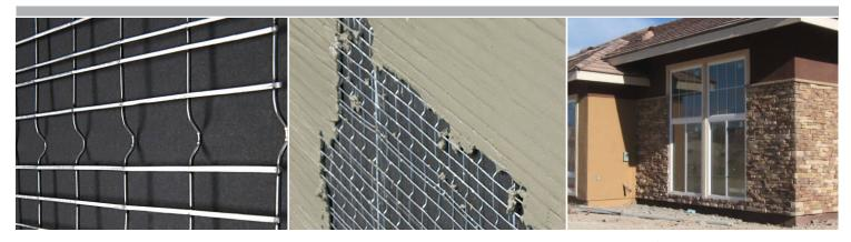
**Structa MEGALATH** is a self-furring welded wire lath for use as an alternative to 3.4 lb/yd² diamond mesh metal lath specified in ASTM C847 and for use as an alternative to 1.4 lb/yd² woven wire lath as specified in ASTM C 1032. **MEGALATH** is the heaviest and strongest welded wire lath available in rolls today. At 1.95 lb/yd², **MEGALATH** can be installed 24" OC over open framing and was engineered to meet weight requirements for architectural stone product installations.
