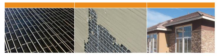
Structa Mega Lath is a self-furring welded wire lath for use as an alternative to 3.4 lb/yd² diamond mesh metal lath specified in ASTM C 847 and for use as an alternative to 1.4 lb/yd² woven wire lath as specified in ASTM C 1032. Mega Lath is the heaviest and strongest welded wire lath available in rolls today. At 1.95 lb/yd², Mega Lath can be installed 24" OC over open framing and was engineered to meet weight requirements for architectural stone product installations.
